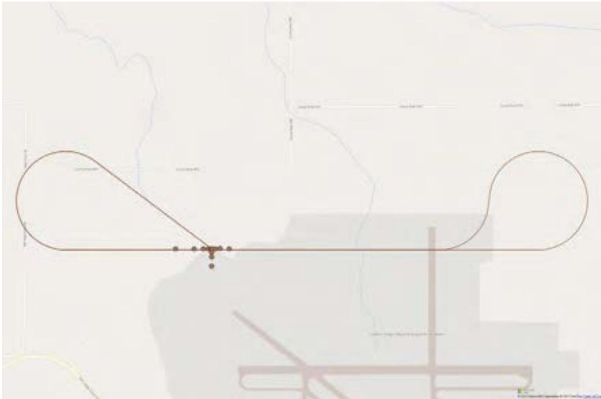
Figure 6. Flyover Flight Pattern (Empty and MTOW)
