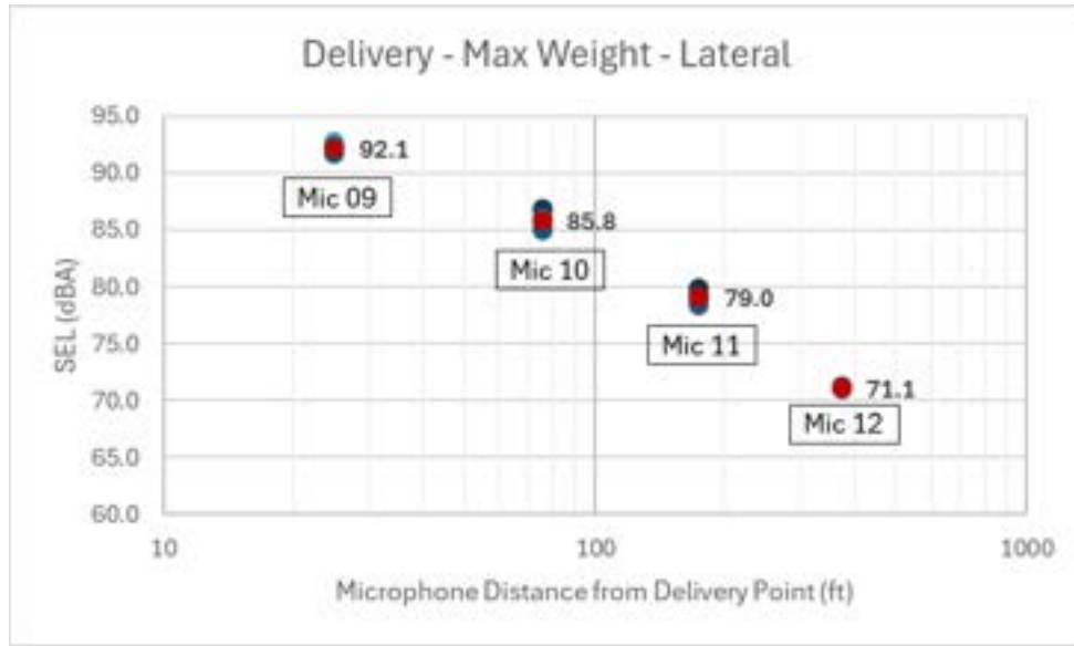
Figure 17. Range of MK30 Averaged A-Weighted SELs from Delivery at Max Weight – Lateral
