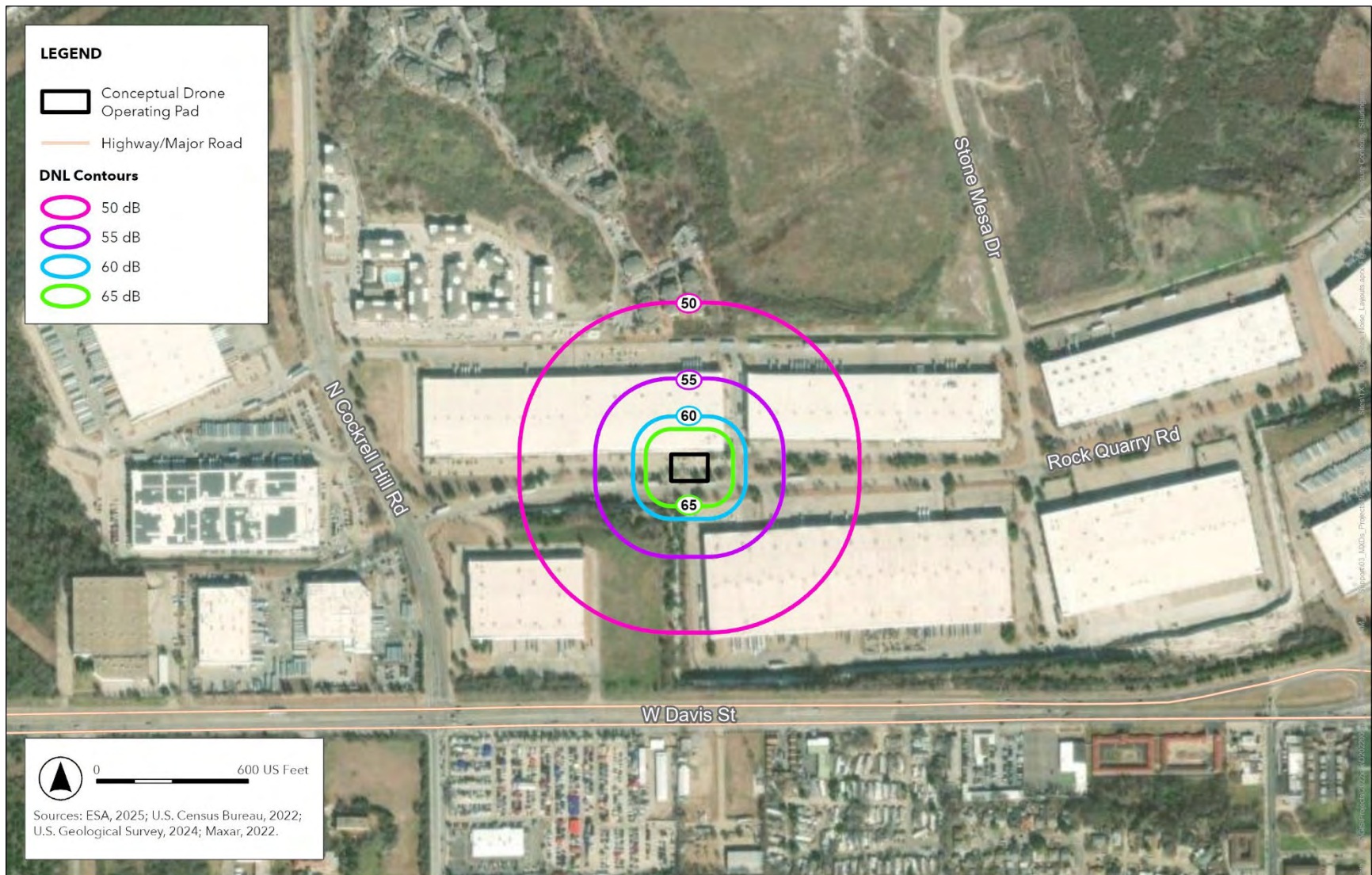
Figure E-5 Noise Exposure Contours – STX3 PADDC
