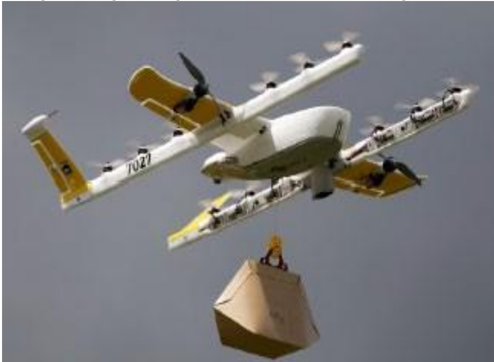
Figure 2. Wing Hummingbird Unmanned Aircraft with Package Attached
