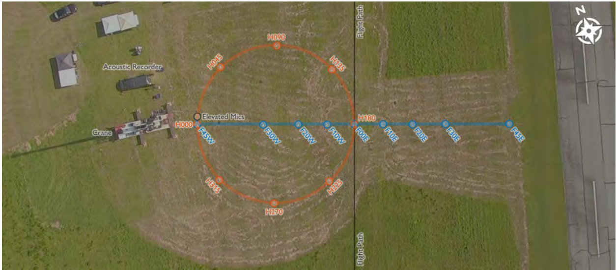
Figure 1. Microphone locations for hover measurements shown in orange when FTXM600P UA hovered above the origin.
