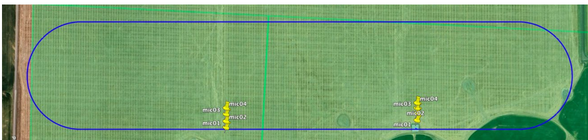
Figure 3: MK27 Flight Path with Microphone Locations
