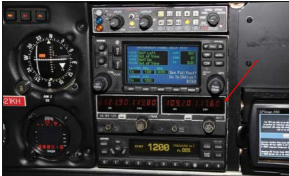
Figure 4: Aircraft Instrument Panel with VHF Communications Transceiver
