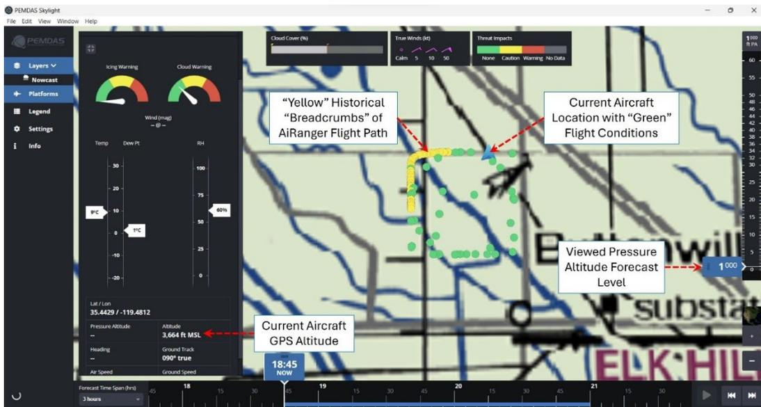
**Figure 20 ASAPS Cloud Warnings Displayed on Skylight (14 Jan 2024)**
