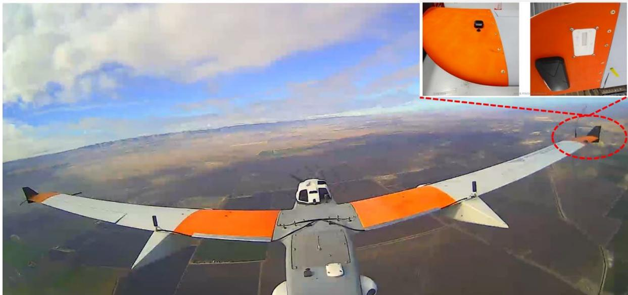
**Exhibit D3. ASAPS Installed on AiRanger's Right Wingtip**
