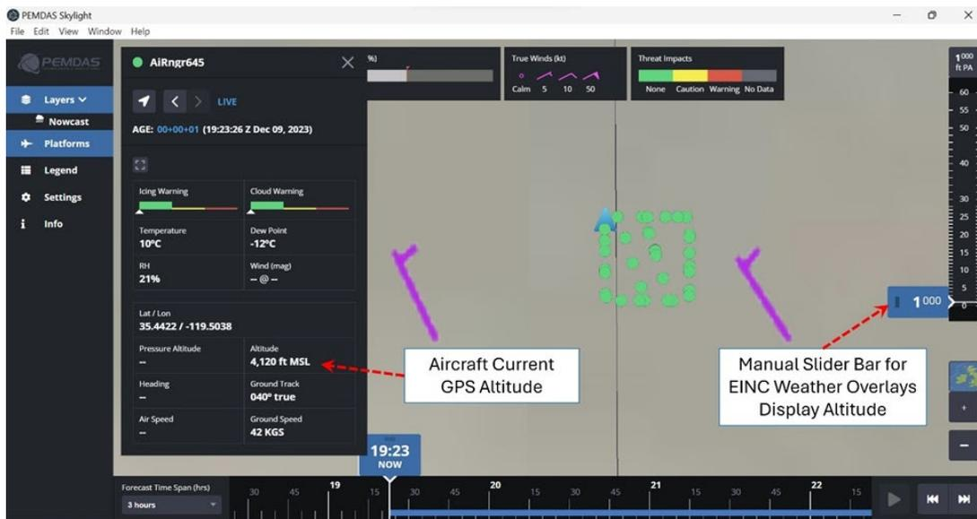
**Figure 33 Skylight Altitude Adjustment Operation**
