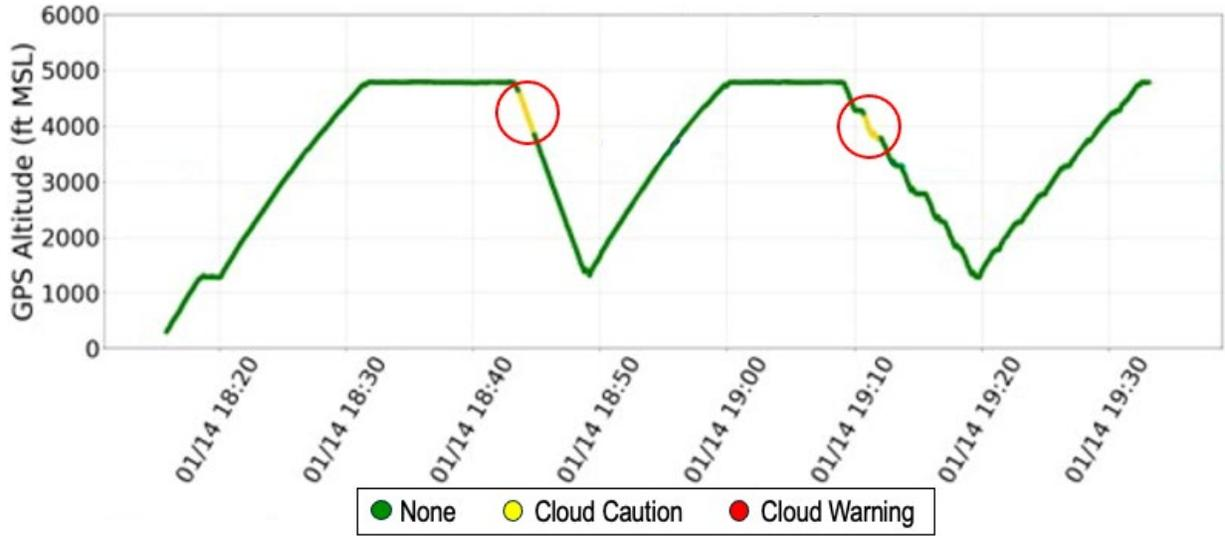
**Figure 18 ASAPS Altitude Color-Coded Cloud Warnings (14 Jan 2024)**
