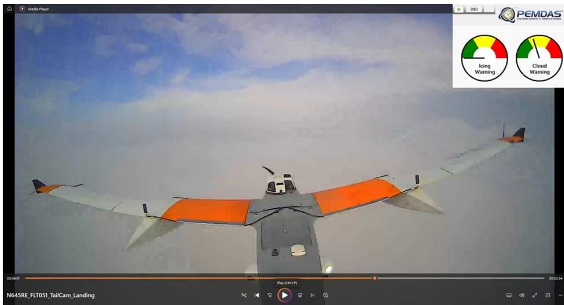
**Figure 23 AiRanger Tail Camera Video and ASAPS Cloud Caution Display During Descent**
