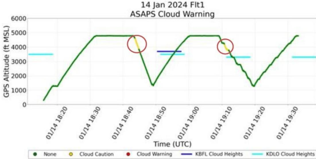
**Figure 15 14 January 2024 Flight 1 ASAPS Altitude Color-Coded Cloud Warnings**
