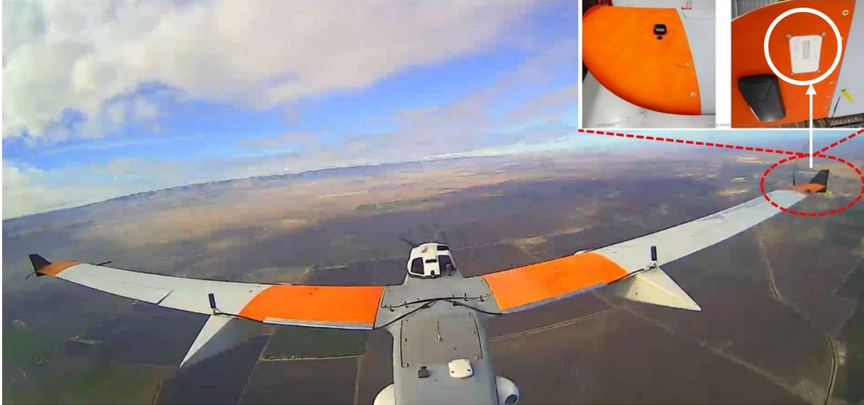
**Figure 5 ASAPS Installed on AiRanger’s Right Wingtip**
