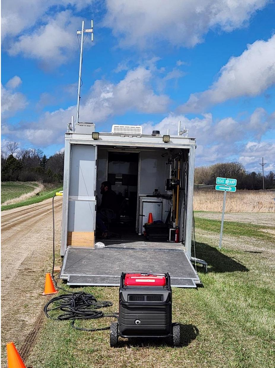
**Figure 21.** uAvionix SkyLink GRS Installed on NPUASTS Mobile Command Trailer at Niagara, ND
