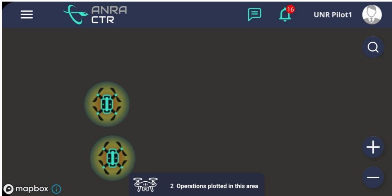
Figure 25: Screenshot of ANRA CTR app (mobile) provided NRID capabilities, depicting two BRID equipped drones
