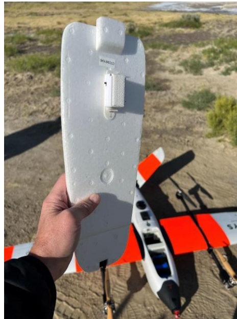
Figure 9: Sentaero hatch with BRID module mounted on underside of hatch
