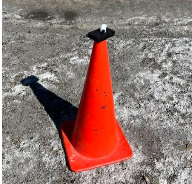
Figure 20: Ground based, stationary BRID module with attached battery pack
