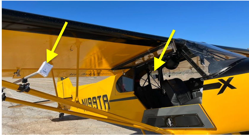
Figure 7: Externally mounted EFB receiver on the right-wing strut and the other EFB receiver mounted inside the cabin.
