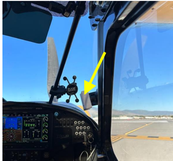
Figure 31: EFB BRID receiver mounted above xCub glareshield on cockpit starboard window.
