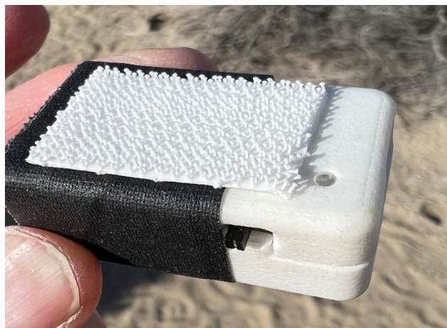
Figure 3: BRID module with Velcro tape to fasten to UAS
