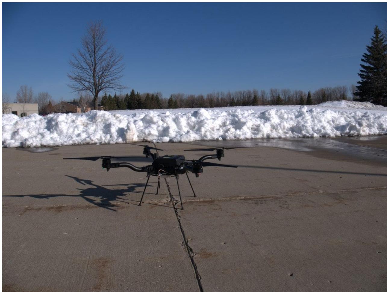
Figure 17: FreeFly Astro with uAvionix muLTElink-5060 ARS Installed Waiting for Launch
